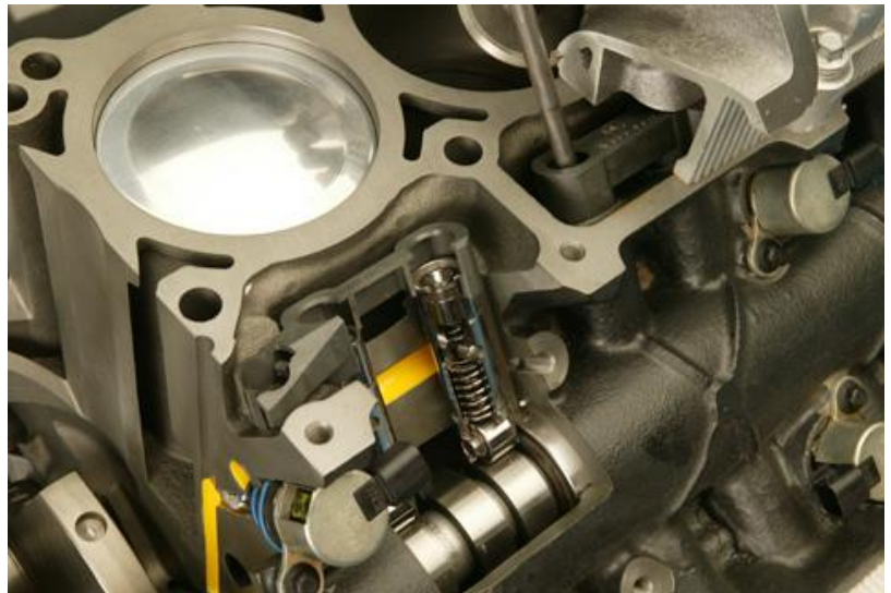
MDS Engine Cutaway(allpar.com)
