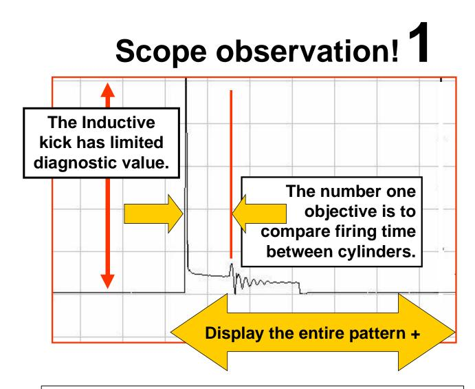
The purpose of the ignition system is not only to ignite the spark in the combustion chamber at the right time, but also to maintain the firing for as long as there is fuel in the combustion chamber.
