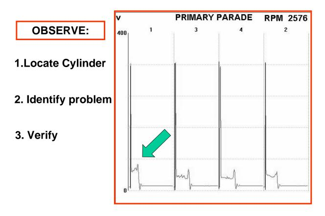
It is now obvious that cylinder # 1 has a poorer conductivity to maintain a spark, compared to the other cylinders.
