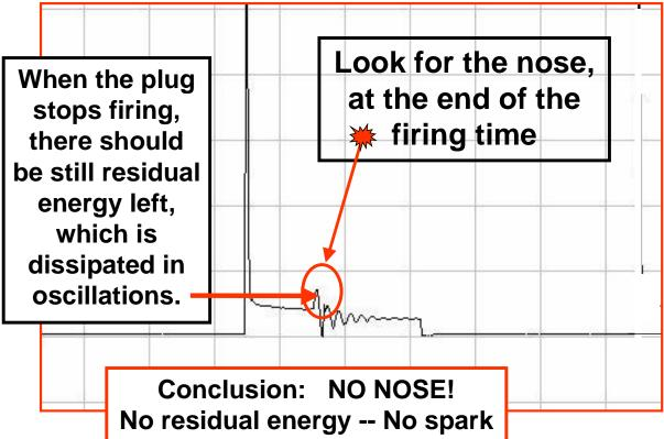
Take a quick look at the upward nose of the first oscillation, which indicates the end of plug firing.
