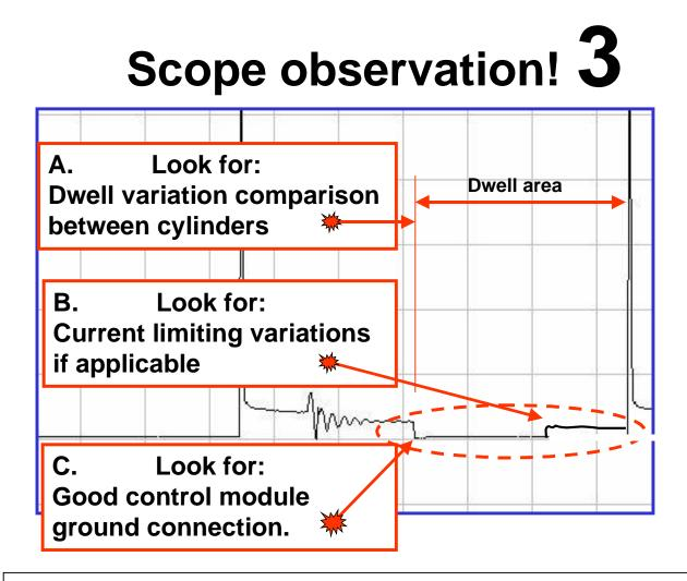
The dwell section is a significant evaluation of module comparison. Since each cylinder has its own coil and driver, make a mental note of any variation that does not occur on the other coils.
