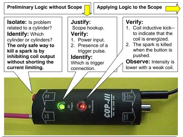
Above description applies to the model COP-II and the COP-III, serving as a preliminary check and a quick way to justify a scope hookup.
