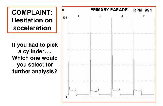
For the "Die-hard Scope Wizard", looking at a scope pattern without KV, feels like diagnosing blind folded. However, that is only a matter of practice and applying the lessons learned from secondary analysis.
